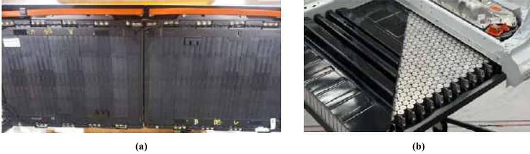
Fig. 1.2 Example of cell configuration in EV: (a) Pouch type; (b) Cylindrical type.
